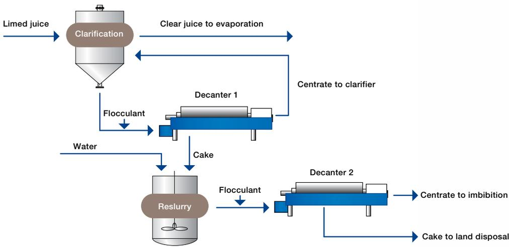
Sugar recovery is maximized by using a system with two decaners. The cake coming out of the first decanter is re-slurried in water in order to wash out the residual sugar. The slurry is then fed to the second decanter.
